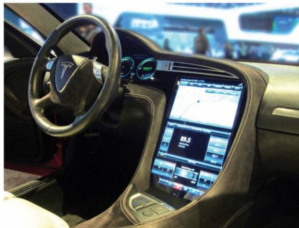
The interior of the Model S features a 17-in infotainment touch screen with 3G/4G wireless connectivity.
